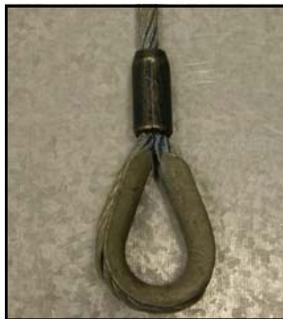
Notice how the thimble in the sling eye above is tight. The pressed metal sleeve is close to the base of the sling eye, and the wires form nicely around the thimble's small diameter.
